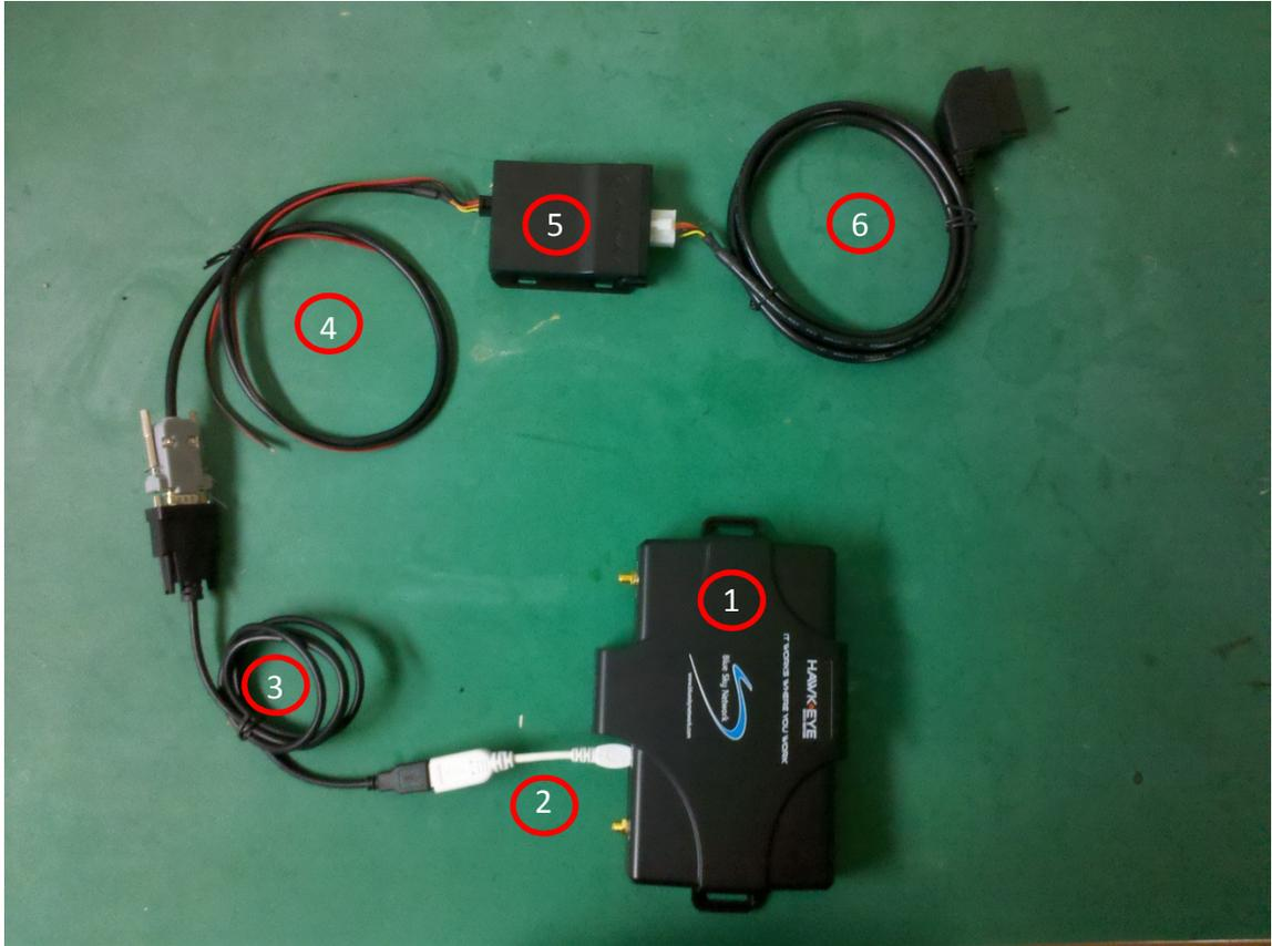
**Figure 1.B:** Using Yamei OBD and its necessary components
