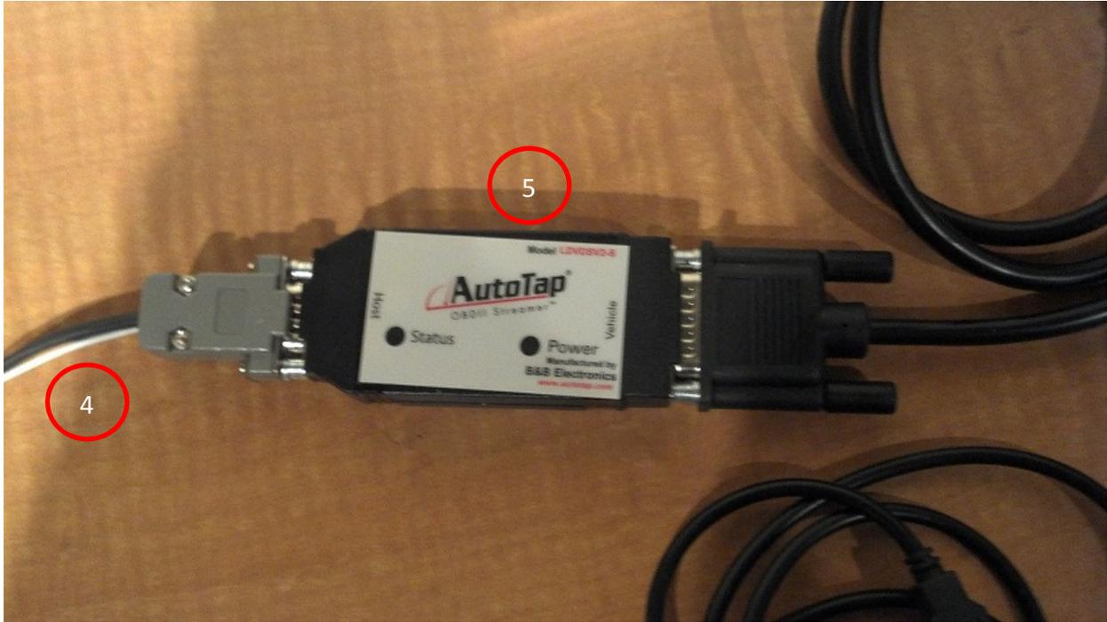
**Figure 5.A Using B&B OBDii Adapter**
