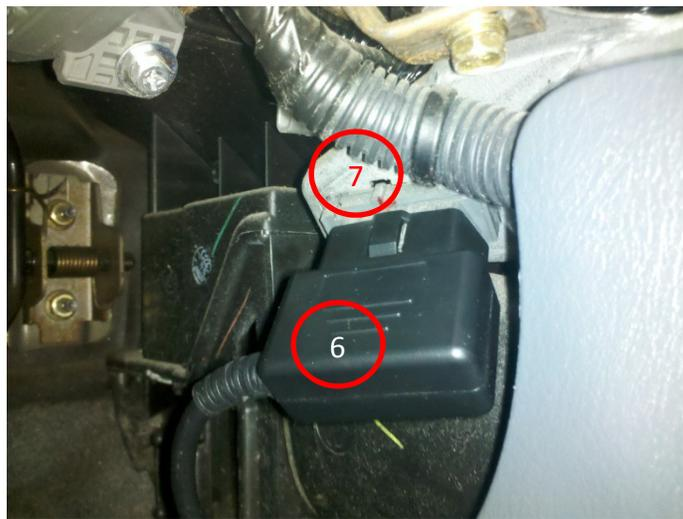
*Figure 8 Connecting OBDii connector*
