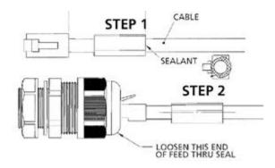
Figure 4-8 Installing Ethernet Cable through fitting
