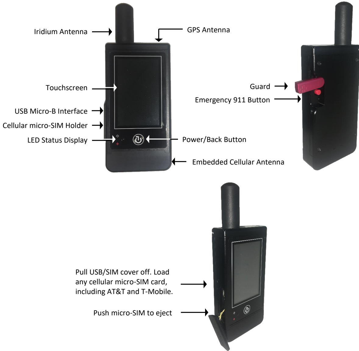
Figure 1: SHOUT 3G Exterior Components
