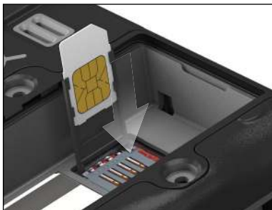
Inserting the SIM card
