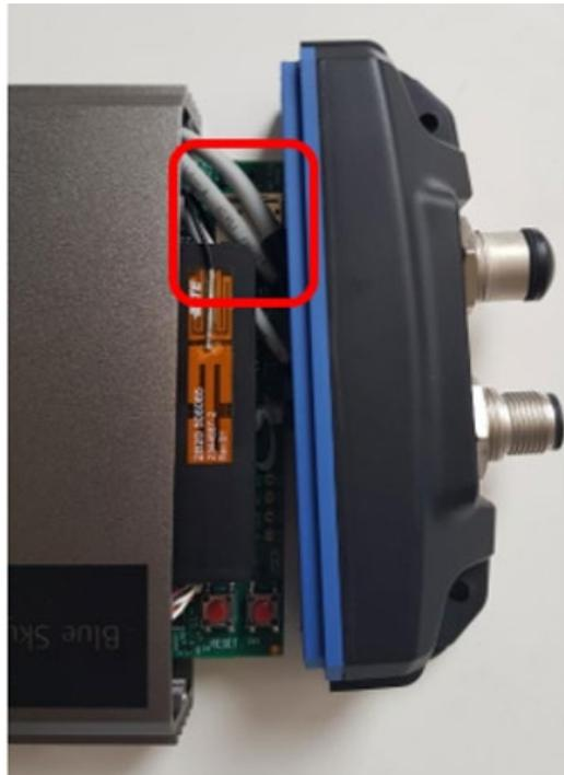
3. Flip the device over to the back panel (where the white label is located) and insert the Iridium SIM card into the slot.
