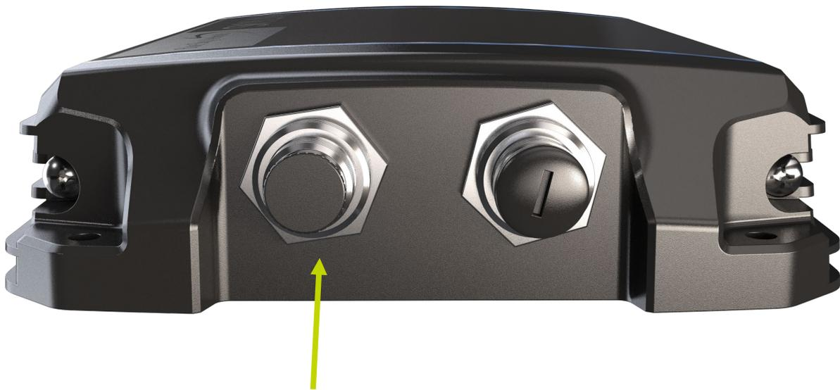
To power on the device, remove the connector cap from the power port located on the bottom panel of the unit. Connect the power cable into the port and the adapter into the appropriate power source (e.g., a wall or vehicle outlet).
