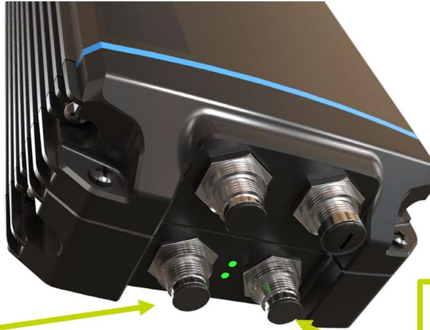
The power connector is on the left-hand side when the logo is facing up.
