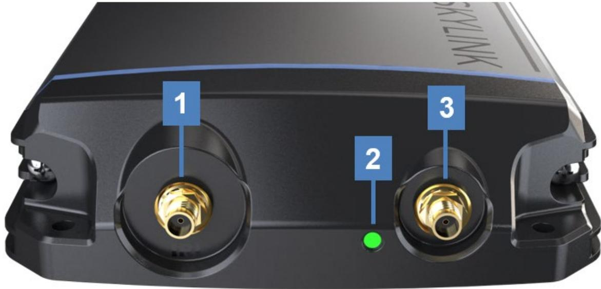
The top panel contains a power LED indicator and 2 connectors for an Iridium and cellular antenna. The descriptions below reference the photo above in accordance with the numerical value.
