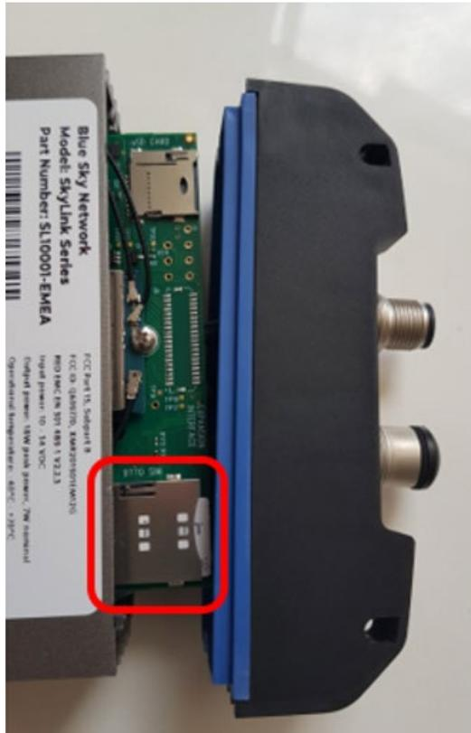
**NOTE:** A micro SD slot is also present behind the connectivity port. Ensure that the SIM cards are placed into the correct holders and not the micro SD slot. If the device does not work after installing the SIM cards, they may be in the wrong slots.
