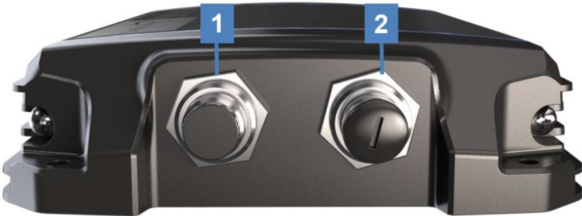
The bottom panel contains a power port and a connectivity port that connects to multiple adapters. The descriptions below reference the photo above in accordance with the numerical value.
