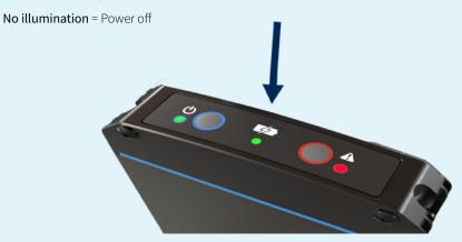
**NOTE:** The Battery Pack has 2 battery cell packs and only one status LED. As a result, status colors may alternate if the cell packs are in different states. For example, if one is charging and the other is done charging, the LED will alternate red and green.
