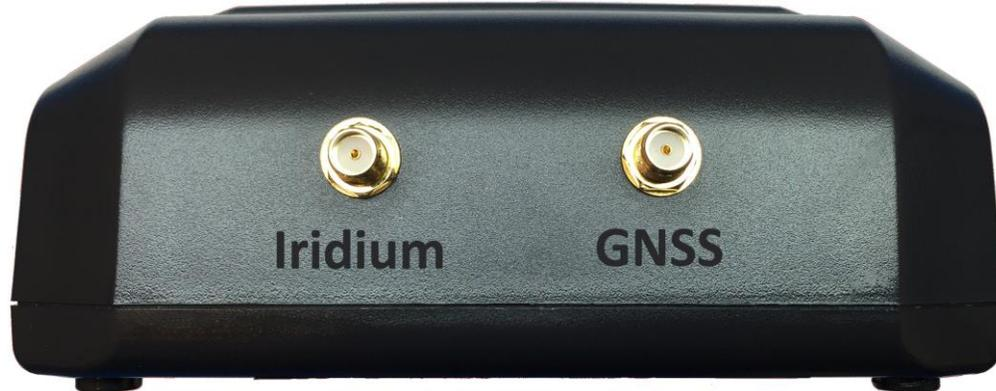
The HawkEye 7200X provides SMA Female antenna connections for both Iridium and GNSS. When connecting an external antenna cable, be sure to tighten the connectors securely by hand, do not over torque the connectors (this could cause internal damage to the device.)
